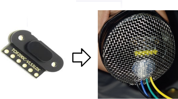
Figure 3: Infrared sensor and the grid placed at the base of the pipe
