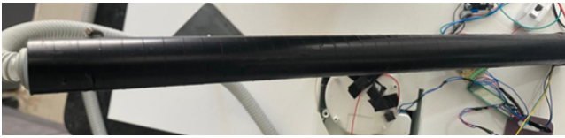
Figure 2: Picture of the mica tube used in the designed sensor system
